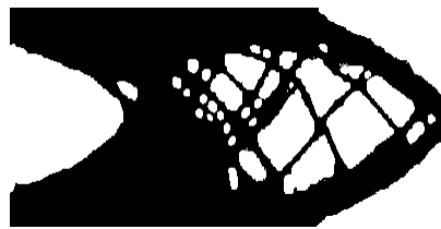
Figure 8. Cantilever beam design using both reference inputs from Figure 3; Compliance: 61.147.
