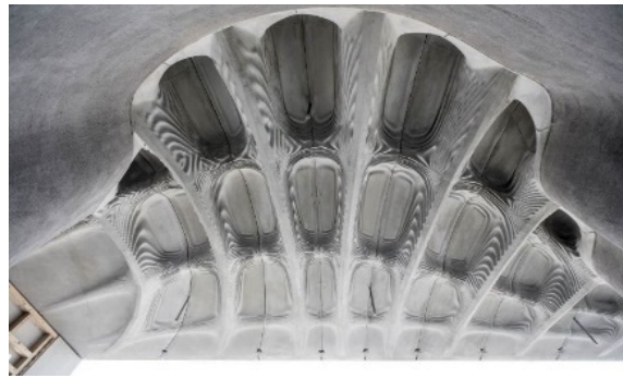
Figure 5. Concrete part formed on a Binder-Jetted tool [38].
