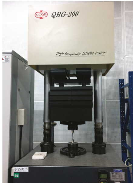
Figure 6. Setup of the fatigue experiments.
