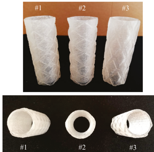
Figure 3. Stent prototypes printed by ACEO and used for the experimental compressive tests: #1 prototype, #2 prototype, #3 prototype.
