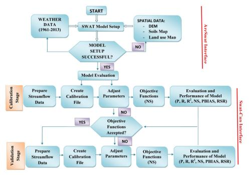
Figure 2. Diagram of SWAT model [48].
