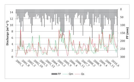
Figure 5. Simulated river discharge (Qs), measured river discharge (Qm) and precipitations (PP) for the Tărlung watershed for the 2001-2010 period.
