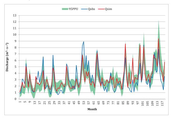
Figure 6. The 95PPU plot between observed and best simulated discharges after the calibration procedure.
