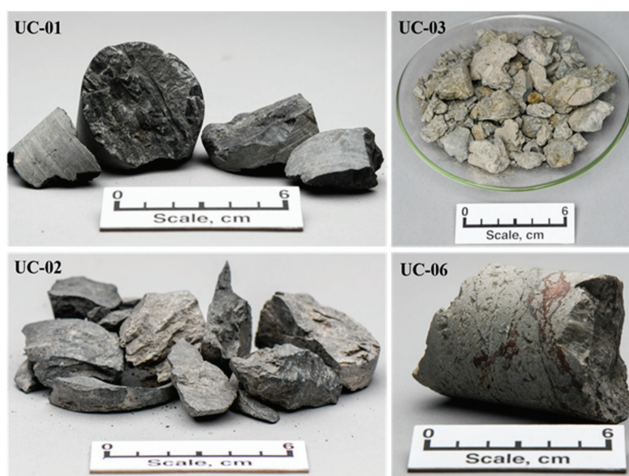
Figure 1. Photographs of as-received underclay core samples examined in this study. Information and descriptions of rock from the core samples are shown in Table 1.
