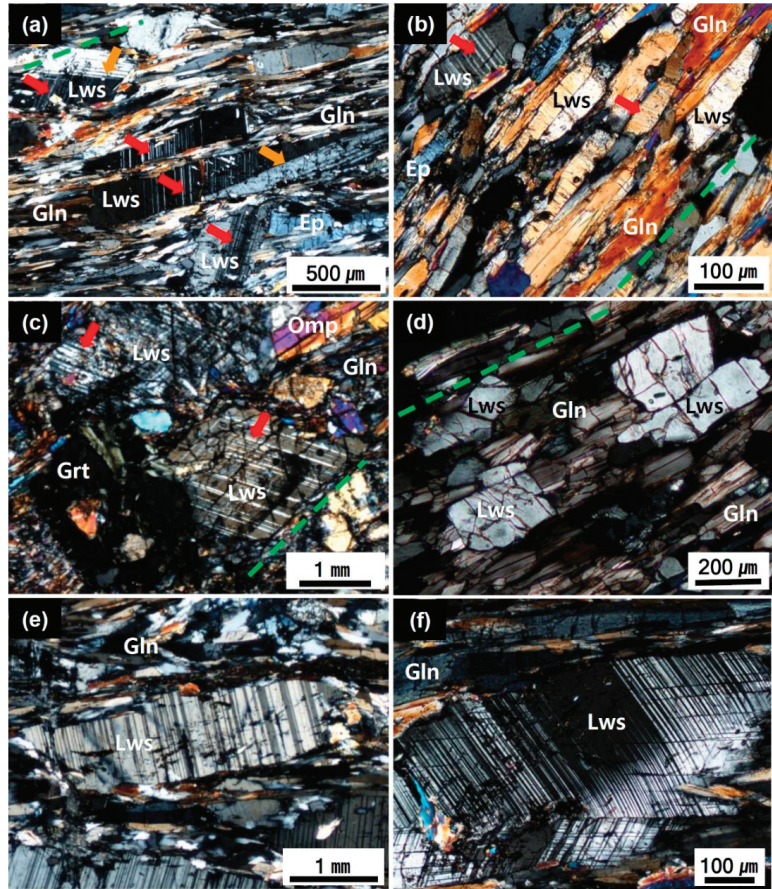
Figure 3. Enlarged photomicrographs of lawsonite blueschist samples. All photos are from thin sections in the x-z plane in cross-polarized light. (a) High lawsonite twin frequency (sample 3034); (b) medium lawsonite twin frequency (sample 3033); (c) low lawsonite twin frequency (sample 2023); (d) very low lawsonite twin frequency and some fracturing in lawsonite (sample 2021); (e) representative polysynthetic twin in lawsonite (sample 3034); and (f) representative deformation twin with curved textures in lawsonite (sample 3034). Some crossed twins can be observed as the second generation of twins, which are horizontal in (f). The green dashed lines indicate the foliations of the samples, and red and orange arrows denote the polysynthetic and deformation twins, respectively. Lws: lawsonite; Gln: glaucophane; Grt: garnet; Omp: omphacite; Ep: epidote.
