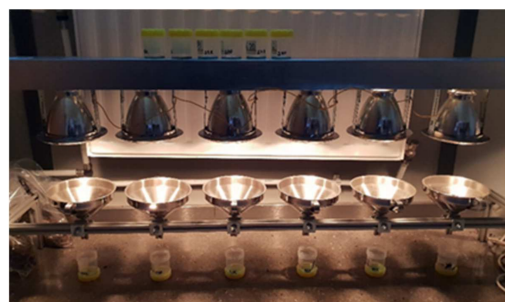
Figure 2. Tullgren funnels utilized for the collection of invertebrates.
