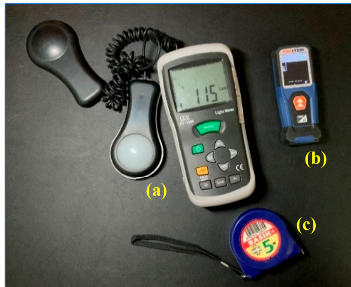
Figure 3. Equipment used in the testing campaign: (a) CEM-DT 1308 lux meter, (b) DEXTER CM30 distance meter, and (c) measuring tape.
