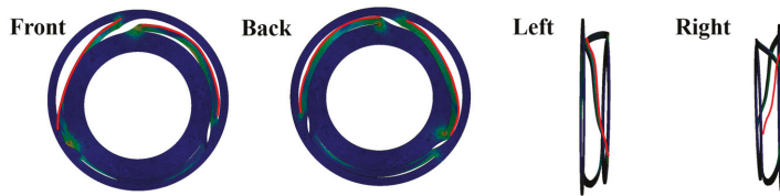
Figure 18. Expected deformation shape (highlighted with red lines) of the spring after the impact.
