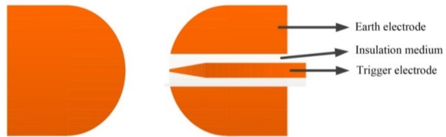
Figure 5. Schematic diagram of the trigger switch.
