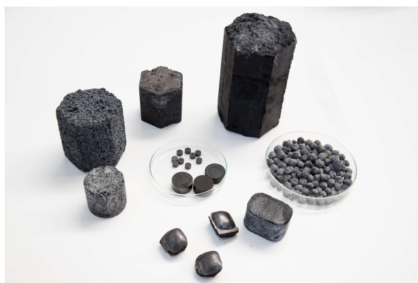
Figure 4. Exemplar of cold-bonded briquettes, agglomerates and pellets produced at VDEh-Betriebsforschungsinstitut GmbH.
