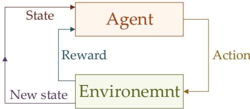
Figure 2. Block diagram of reinforcement learning (RL) control.
