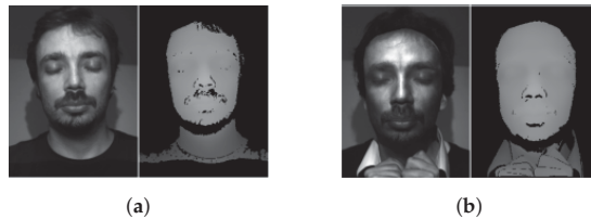
Figure 14. The texture image and its corresponding depth image for (a) a real access and (b) a 3D mask attack: the figure was extracted from [25].
