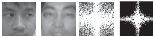
Figure 9. From left to right: a genuine (alive) face, a printed photo attack and their respective 2D Fourier spectra (Figure extracted from [44]).
