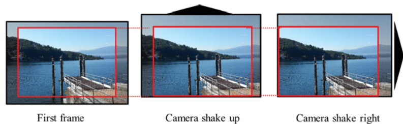
Figure 1. Digital motion video stabilization on subsequent frames. Undesired camera shakes are compensated for in order to have stable contents.
