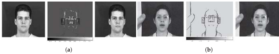
Figure 4. The Optical Flow Lines (OFL) images obtained from (a) a genuine (alive face) presentation with a subtle facial rotation and (b) a printed photo attack with horizontal translation [46]: in (a), the inner parts are brighter than the outer parts of the face, which is characteristic of the motion differences between different face parts. In contrast, all parts of the planar photo in (b) display constant motion.
