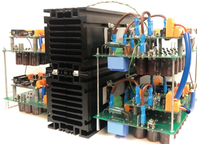
Figure 12. Single MMC leg/phase (four submodules).
