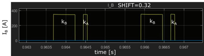
Figure 28. Current of braking choppers ( I_B [A]) vs time [s] for mixed duty cycle (MCD) k_A = 0.1 , k_B = 0.5 (effective duty cycle k = 0.3 ).
