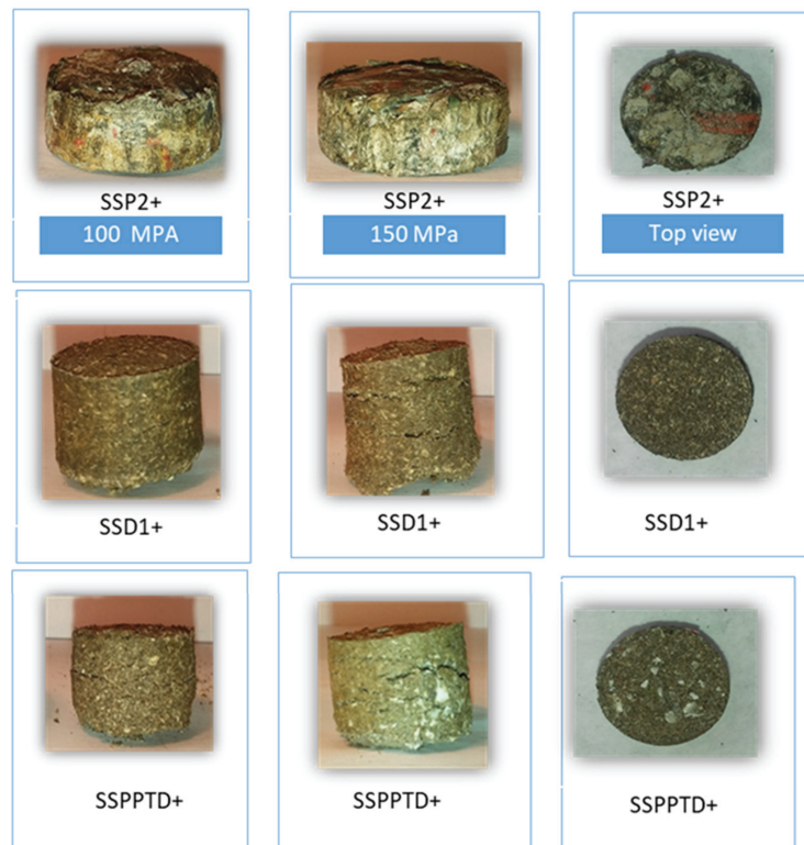
Figure 9. Briquettes of SSP2+, SSD1+, and SSPPTD+ (pressure 100–150 MPa).
