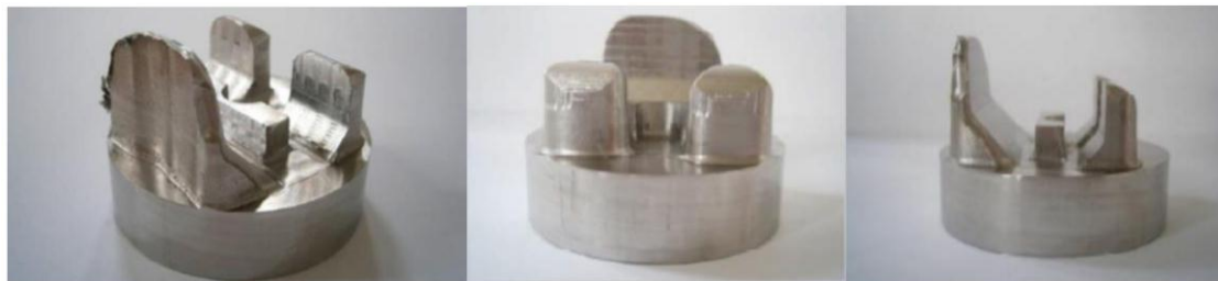
Figure 6. Views of the workpiece after the first machining stage.
