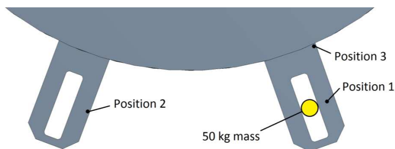
Figure 4. Positions of the dial gauges and of the applied mass.
