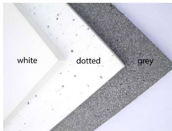
Figure 1. The tested products: A—“white” expanded polystyrene (EPS) (pure), B—“dotted” EPS, and C—“grey” EPS.
