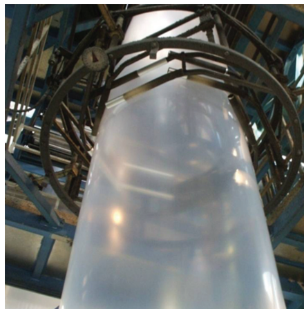
Figure 1. Photo of a bubble for plastic film extrusion. Bubble diameter is 1.5 m.
