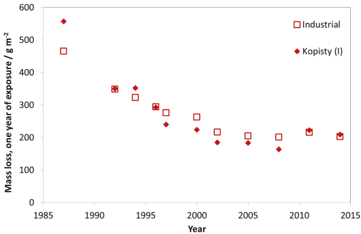
Figure 9. Carbon steel corrosion, average of industrial sites and the industrial site Kopisty.
