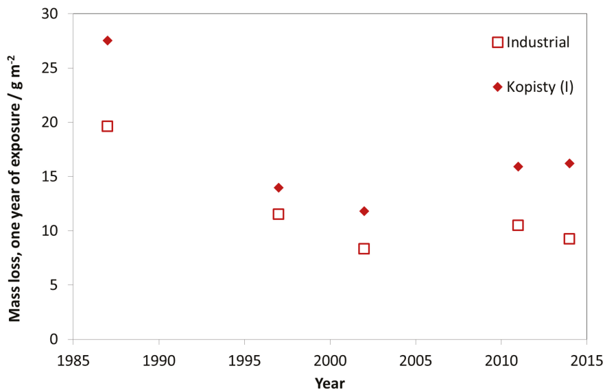
Figure 21. Copper corrosion at industrial sites and the industrial site Kopisty.
