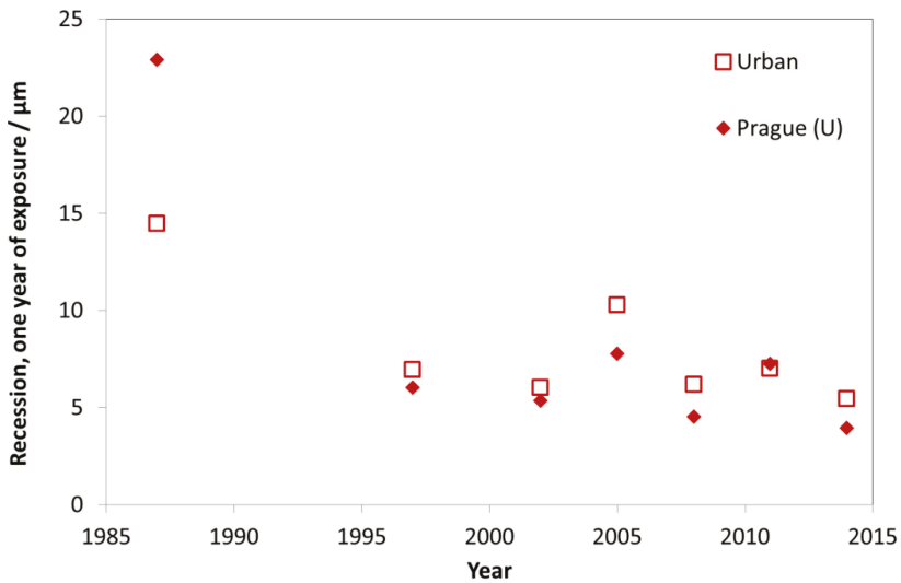
Figure 28. Limestone surface recession at urban sites and the urban site Prague.
