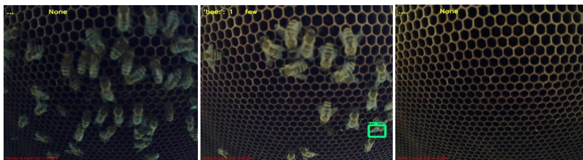
Figure A2. Bee detection with the NVIDIA Jetson Nano using the SSD algorithm, Inception v2 model, for Classes 0, 2, and 3.
