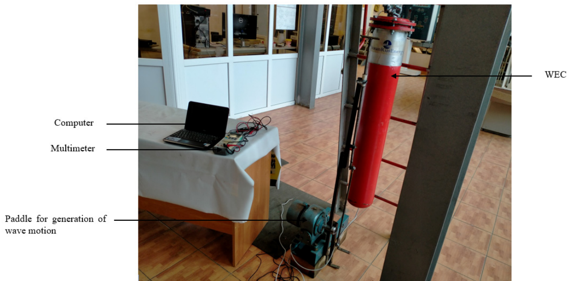
Figure 6. Experimental setup for the point-absorber WEC generator.
