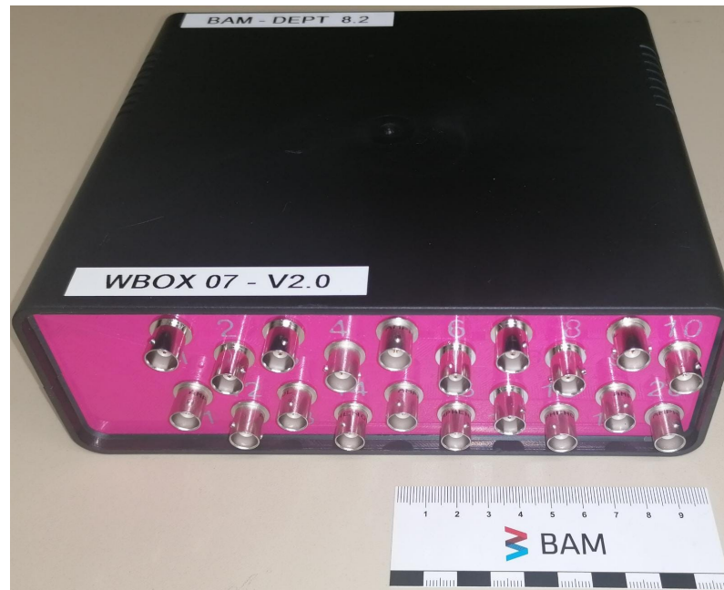
Figure 1. The W-Box. The 3D-printed pink side panel holds 20 BNC transducer connectors.
