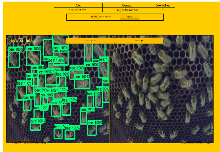
Figure A5. BeeQ RMS web interface to the swarming detection service. It takes as the input uploaded images and performs the offline detection process, illustrating the results.
