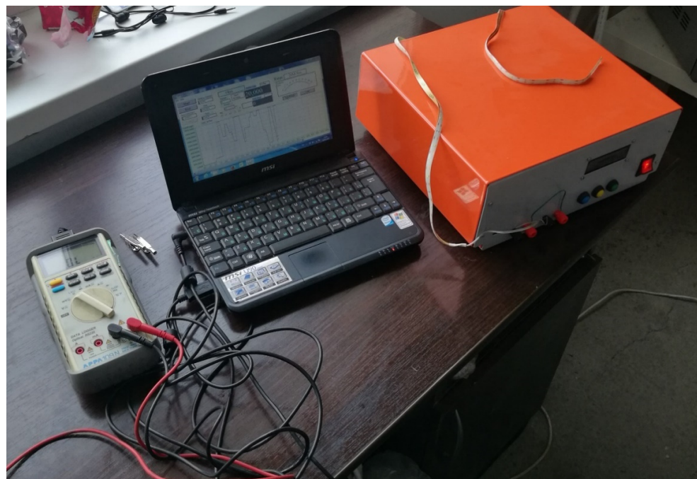
Figure 4. Experimental setup made up of a (from left to right) multimeter, laptop computer and the newly built WEC emulator.
