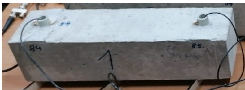
Figure 14. Concrete beam of 40 \text{ cm} \times 10 \text{ cm} \times 10 \text{ cm} and two embedded ultrasonic sensors (S0807 from ACSYS, as used in [11,13,18,19]).
