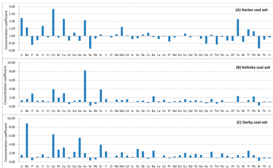
Figure 5. Concentration coefficients of trace elements in the coal ashes studied. (A) Harlan; (B) Kellioka; (C) Darby. Concentration coefficients (CC) are the ratio of the trace-element concentrations in the coal ash samples vs. world coal ash reported by Ketris and Yudovich [26].
