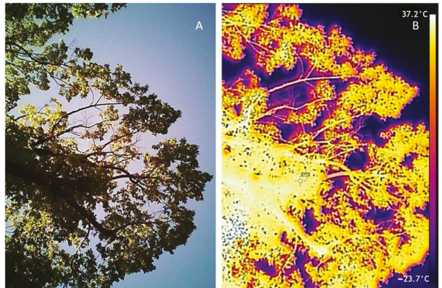
Figure 3. Example of a visible (RGB) image (A) and the corresponding infrared thermal image (B) from an Elm tree taken using the integrated camera on top of a moving vehicle.
