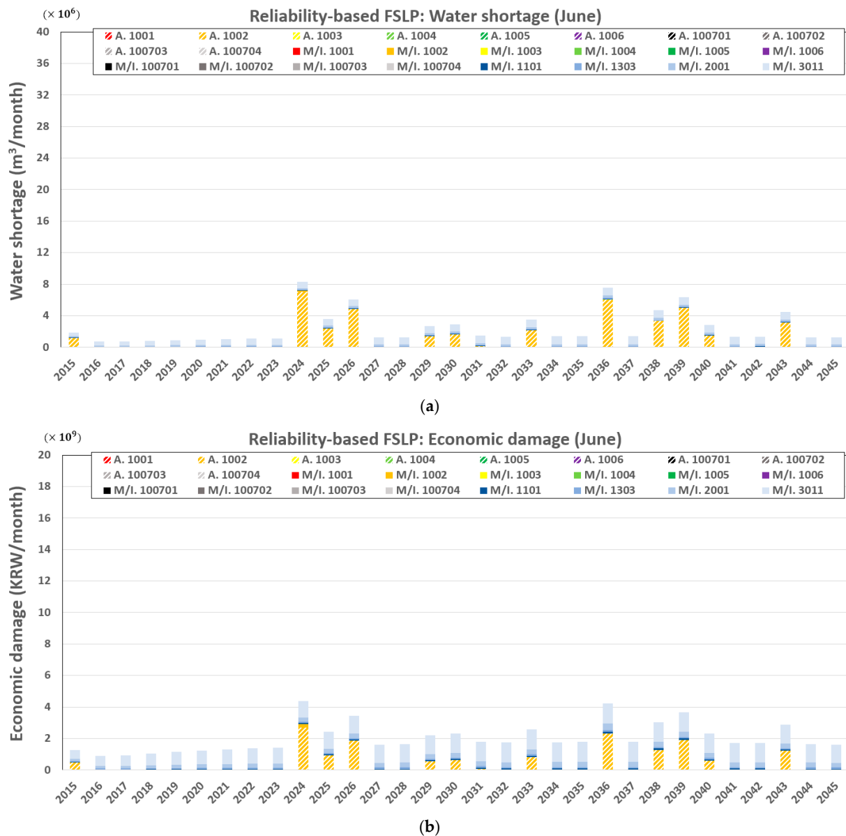
Figure 12. Water allocation simulation results obtained using reliability-based full-step linear programming (FSLP). (a) Water shortage and (b) economic damage.
