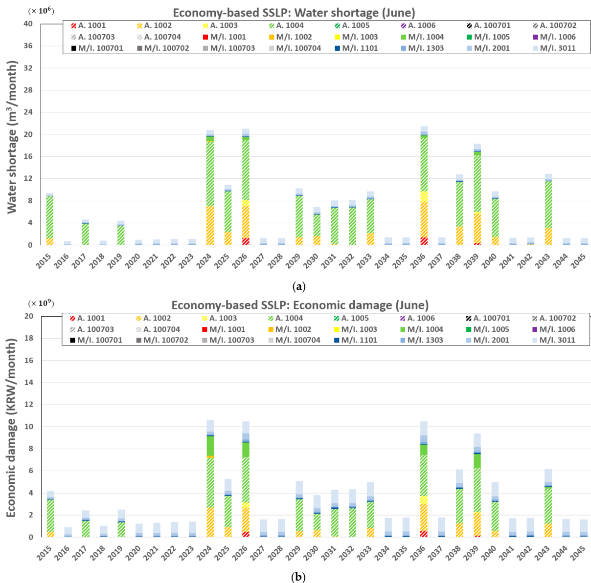
Figure 11. Water allocation simulation results obtained using economy-based single-step linear programming (SSLP). (a) Water shortage and (b) economic damage.
