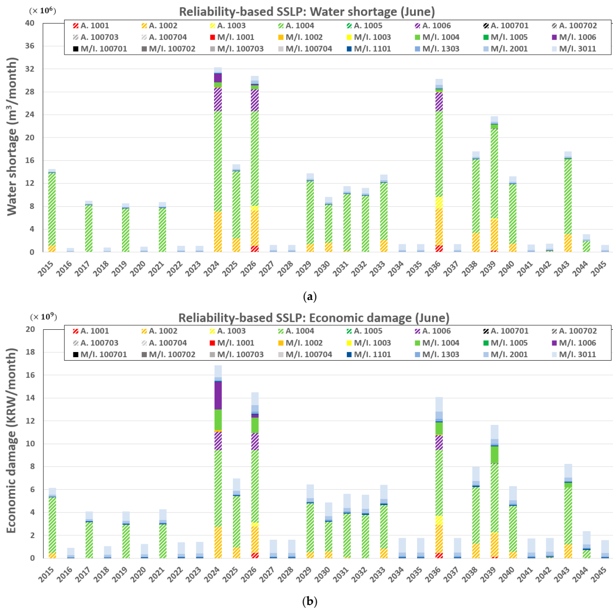
Figure 10. Water allocation simulation results obtained using reliability-based single-step linear programming (SSLP). (a) Water shortage and (b) economic damage.
