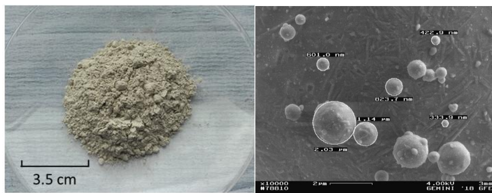
Figure 3. Fly ash powder (left) and SEM analysis (right).
