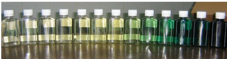
Figure A1. The solution colour changes in the course of molybdenite flue dust leaching. It first became pale yellow (right), then turned into green, and finally dark blue (left).
