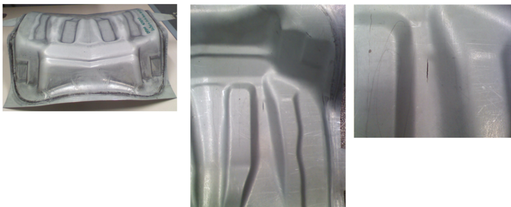
Figure 11. EHF formed part with splits in the areas of maximum strain.
