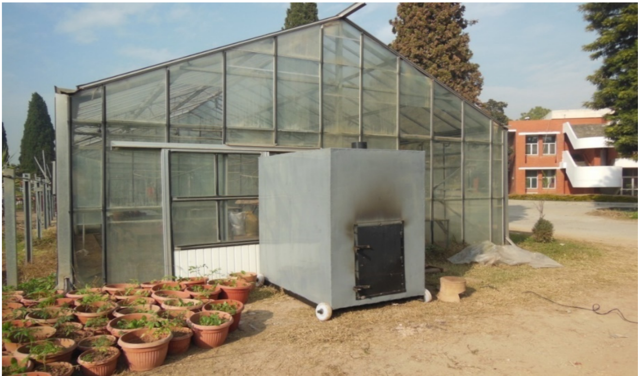
Figure 5. Pretesting of the biomass furnace at NARC.
