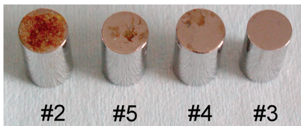
Figure 5. Uniform corrosion salt fog test, according to ASTM B 117-97. Samples #2-1.4427 So, #3-1.4435/316L, #4-316LUGim and #5-316L Val.
