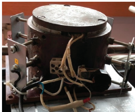
Figure 2. The mold used to obtain material samples by hot pressing [30].
