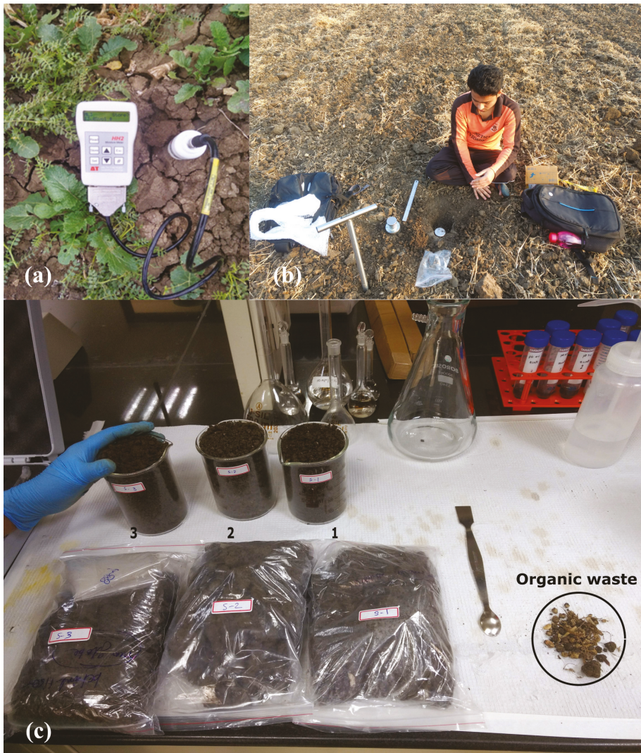
Figure 3. Measurement of soil moisture using (a) ML3 sensor and (b) Collection of soil samples in the field. Photograph (c) Shows the sample processing in the laboratory for oven drying to calculate soil moisture.
