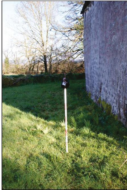
**Figure 2.** The data acquisition process in archaeoastronomy does not involve any kind of disturbance to the archaeological or heritage sites. The picture shows a common procedure for the measurement of a built structure, in this case a Romanesque church in Galicia, Spain. The technique involves deriving a parallel line to the wall to be measured with two rods. © A.C. González-García.
