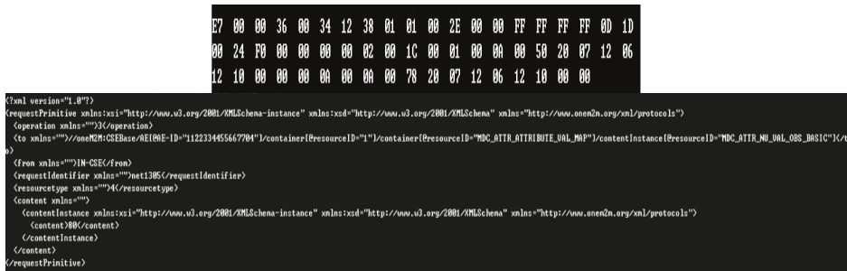
Figure 19. Captured screens of registration (Conversion of an ISO/IEEE 11073 Present (Store Sensing Data) Request message into a oneM2M Update primitive Request message).
