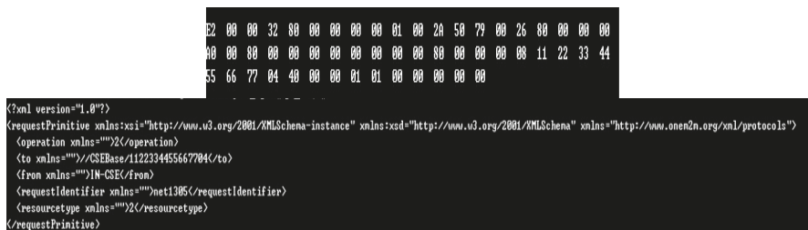
Figure 15. Screen captures of connection establishment (Conversion of an ISO/IEEE 11073 Association Request message into a oneM2M Retrieve primitive Request message).
