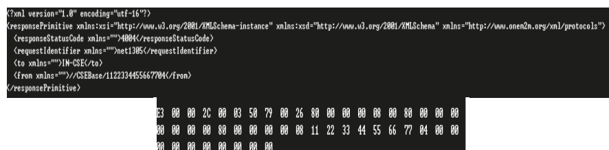
Figure 16. Screen captures of connection establishment (Conversion of a oneM2M Retrieve primitive Response message into an ISO/IEEE 11073 Association Response message).
