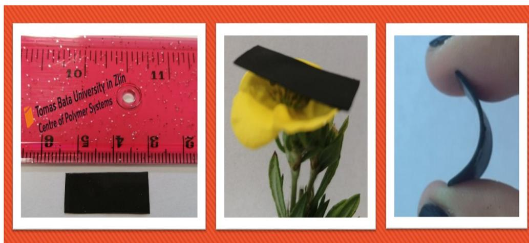
**Figure 3.** Digital photograph of PP nanocomposite embedded with  $\text{MnFe}_2\text{O}_4$  spinel ferrite nanoparticles and reduced graphene oxide (RGO) as nanofillers.
