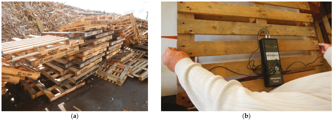
Figure 1. Views on the storage of discarded pallets in Kronospan s.r.o., Zvolen (a), and on the determination of the modulus of elasticity ( MOE_d = \text{density} \times \text{speed of ultrasonic waves in the longitudinal direction}^2 ) of slab in pallet by the ultrasonic timer Fakopp (b).
