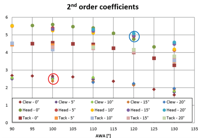
Figure 18. Plots of second order coefficients vs. AWA at different values of \Delta\alpha_g .
