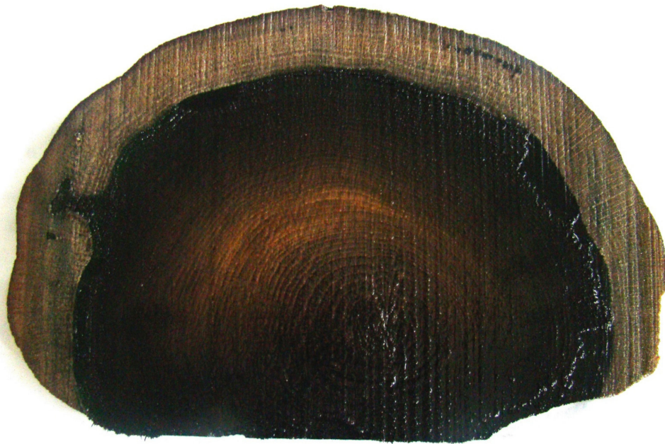
Figure 1. Slice of medieval waterlogged oak excavated from the Lednica Lake, in the Wielkopolska region, Poland, with a severely degraded, soft and light outer ring of sapwood (the loss of wood substance of about 70–80%) and a better-preserved, hard and much darker central part of heartwood (the loss of wood substance of about 10–20%) [35].
