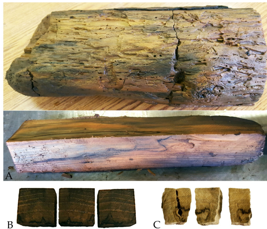
Figure 3. Highly degraded waterlogged elm wood excavated from the Lednica Lake, the Wielkopolska region, Poland (the loss of wood substance was about 70–80% with highly reduced cellulose and hemicelluloses content [42]); (A) part of a log shortly after excavation (upper photo) and cutting (lower photo); (B) untreated waterlogged elm samples (completely filled with water); (C) untreated samples shrunken upon air-drying.
