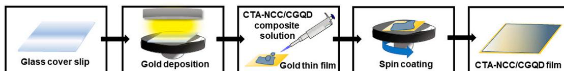
**Figure 1.** Preparation of hexadecyltrimethylammonium bromide (CTA)-nanocrystalline cellulose (NCC)/carboxyl-functionalized graphene quantum dots (CGQD) thin film.
