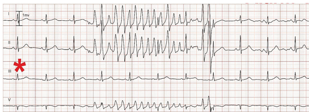
Figure 5. False alarms for ventricular fibrillation. As noted by the *, in lead III, this patient is in a normal sinus rhythm. This particular manufacturer requires a clean ECG signal in at least two ECG leads. Figure from the ECG Monitoring Research Lab, UCSF School of Nursing.
