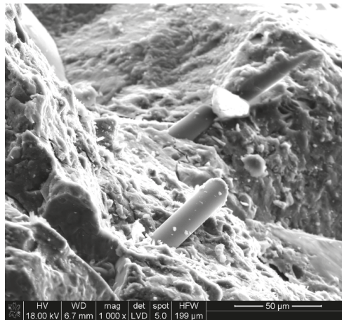
Figure 19. RPC microstructure. Visible parallel arrangement of basalt fibers.
