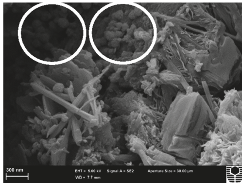
Figure 18. SEM image of 4% nano- \text{Al}_2\text{O}_3 by weight of cement paste hydrated up to 7 days. Reprinted with permission from [107]. Copyright© 2014, Elsevier B.V.
