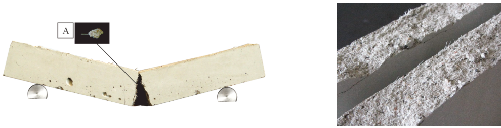
Figure 15. Typical failure modes for specimens [38] with MasterFiber 401 (PVA). (A) Images of the pull-out fracture face of a fiber.
