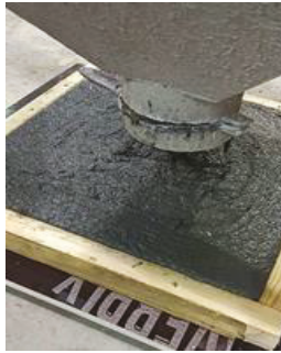
Figure 2. Plate casting direction.
