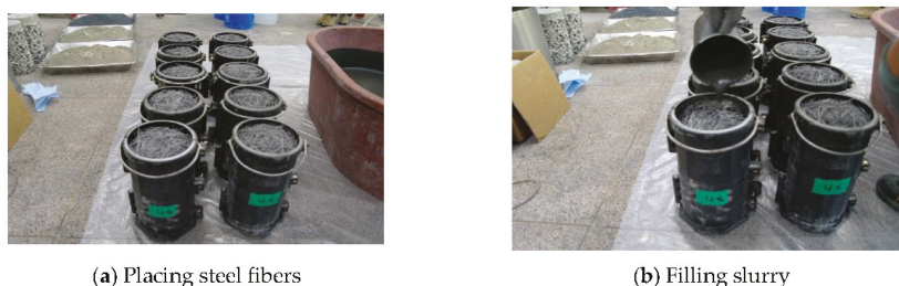
Figure 2. Fabrication of specimens.
