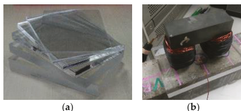
Figure 4. (a) Acrylic plates used in the experiment and (b) experiment set up of an effective depth test.
