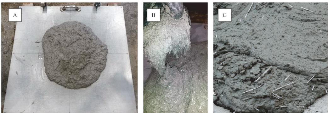
Figure 5. (A) Slump experiment for MasterFiber 401 (PVA). (B) Fresh concrete with MasterFiber 401 (PVA). (C) Fresh concrete with MasterFiber 235 SPA (PP).
