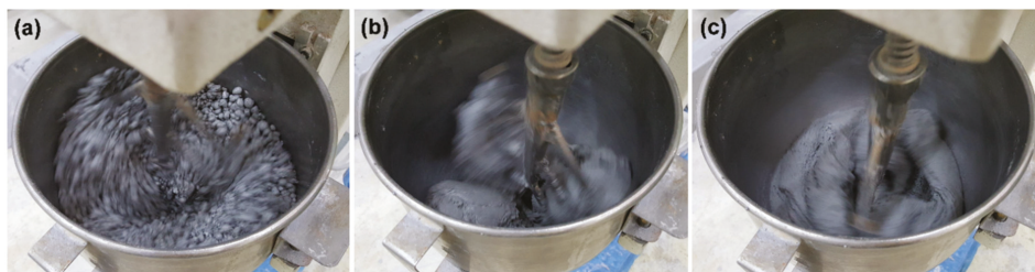
Figure 2. Manufacturing process of UHPFRC: (a) formation of small grains by local agglomeration; (b) agglomeration of small grains into large lumps; (c) dispersion after solid-suspension transition.
