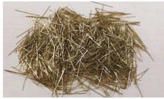
Figure 1. Straight steel fibres used in research.
