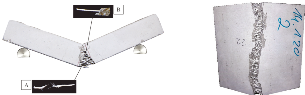
Figure 14. Typical failure modes for specimens [38] with MasterFiber 235 SPA (PP). (A) Images of the tensile fracture face of a fiber. (B) Images of the pull-out fracture face of a fiber.
