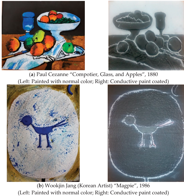
Figure 1. Tactile 3-D printed reproductions in 2.5D model of works (courtesy of Luis Cavazos Quero, Ph.D. student, Dept. of Electronic, Electronic, and Computer Engineering, SungkyunKwan University).
