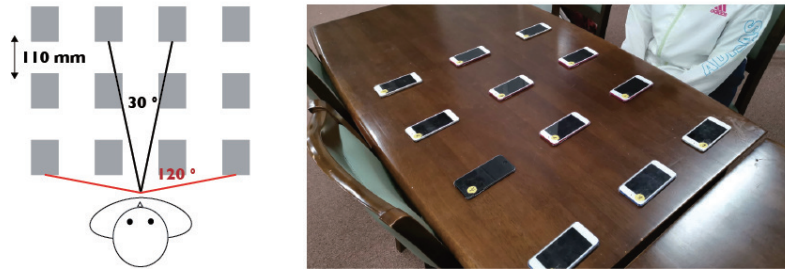
Figure 6. The state of experiment: The subject sat on the chair and described the content and position of the audible cards laid out in front of them.
