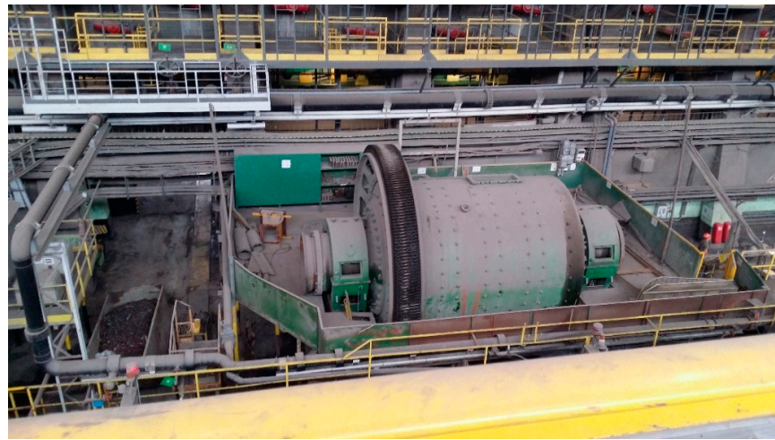
Figure 1. Ball mill of the primary milling stage with the visible gear ring.
