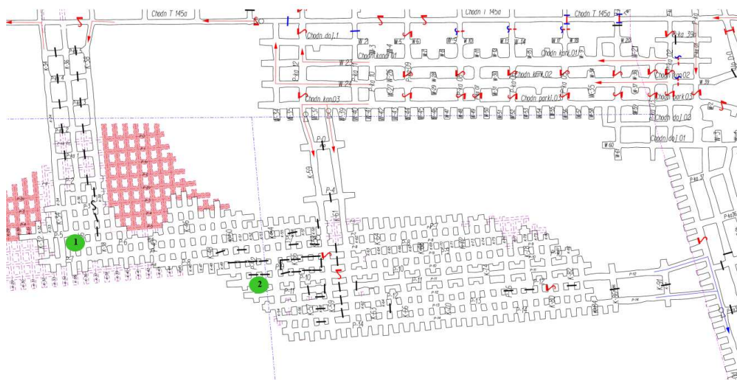
Figure 9. Map of investigated part of mine with fresh and used air stream flow and sensors location.
