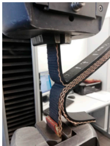
Figure 7. Delamination between ply 1 and ply 2.
