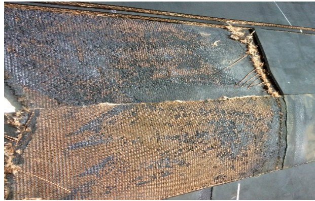
Figure 12. Roughened ply in the splice on belt type EP 1800/5.
