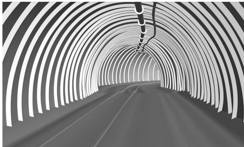
Figure 4. Geometry of the numerical mode—an ‘inside’ view of a straight section of a mine gallery before a bend.
