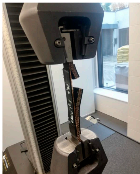
Figure 9. Schematic view of the specimen prepared for splice shear strength tests.
