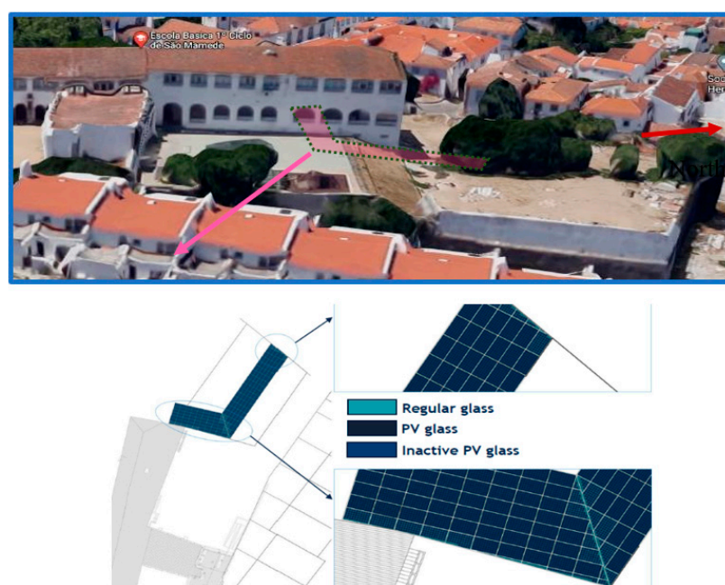
Figure 16. Aesthetic photovoltaic pergola solution proposed by ONYX for S. Mamede School.
