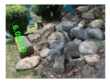
**Figure 20.** Close up of Set #2 meshed 3D CG reconstruction, with measurements on long rectangular prism-shaped rock that was used as reference.
