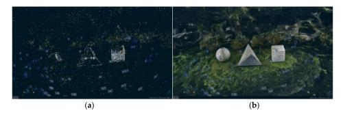
Figure 9. The sparse point cloud (a) and dense point cloud (b) of a scene.
