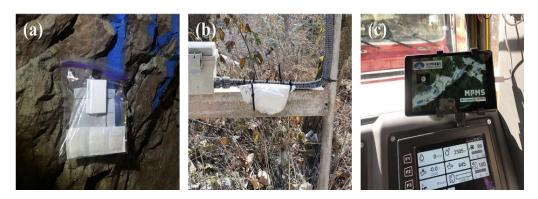
**Figure 2.** Example of Bluetooth beacon (Beacon i3) and Tablet PC (Galaxy A 8.0) installed for log data collection: (a) tunnel wall on the transport route; (b) near the crusher at the crusher; (c) windshield in the driver's seat of the truck.
