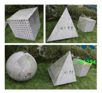
**Figure 14.** Mesh reconstructed 3D CG model of the monuments. The third picture (bottom) shows the measured side of cube monument when using 100 images.
