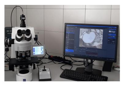
Figure 3. Microscope Zeiss Axio Imager Z 2m.
