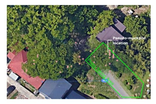
**Figure 18.** GNSS location of camera positions as logged by a smartphone (red dots) of the experiment on a pseudo-muckpile.
