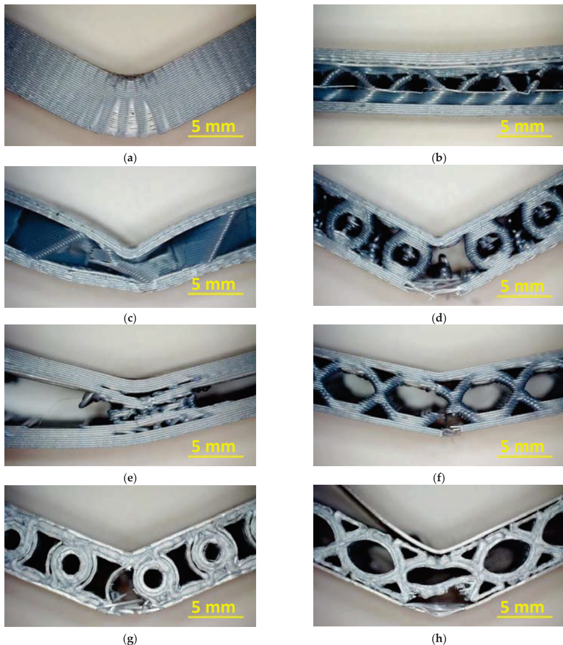
Figure 2. Microscopic images taken after three-point bending tests of samples with different infill patterns: (a) LN100; (b) GY15; (c) OC15; (d) ZHR100; (e) LP100; (f) EW100; (g) ZHR100 printed on the long edge; and (h) EW100 printed on the long edge. Sample LP100, printed on the long edge, will be shown later.
