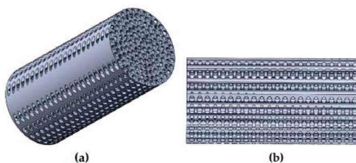
Figure 8. Drawing (a) and cross-section (b) of the catalyst made in the SolidWorks software.
