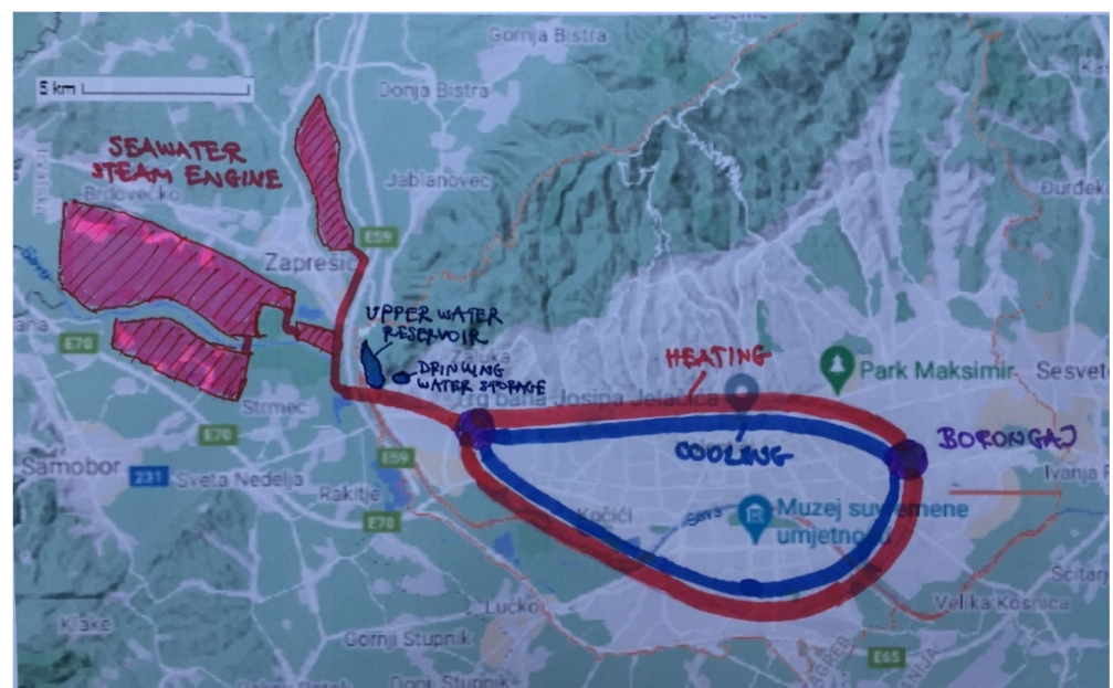
Figure 3. Layout of the collector fields of SSE technology (which uses Sava River as input water) and distribution loops of heating and cooling for the city of Zagreb.
