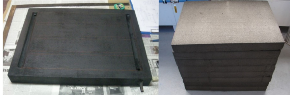
Figure 4. The prototype of the foam glass block with surface treatment ( left ) and raw foam glass plates ( right ).
