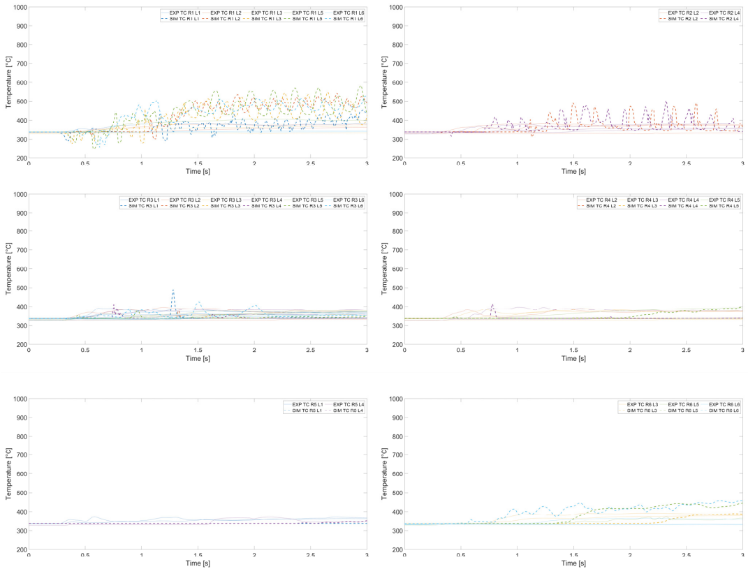
Figure 18. Temperature evolution in S1B for coupled simulations at different radial and axial positions (refer to Table 5).
