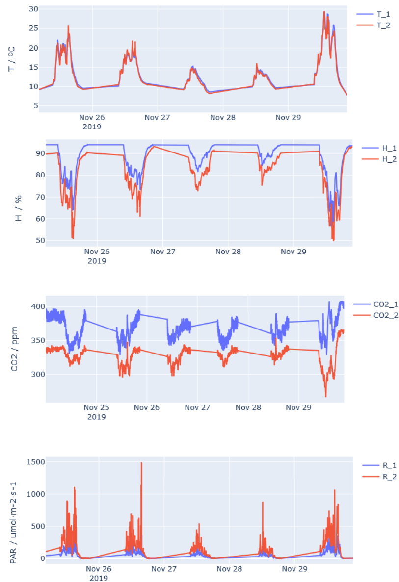
Figure 13. Evolution after planting of temperature, relative humidity, CO 2 concentration and PAR radiation (1: PV glass, 2: conventional glass).
