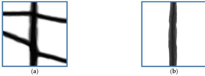
Figure 1. Simulated structures of dimensions 800 nm × 800 nm: (a) branched fiber; (b) single fiber.
