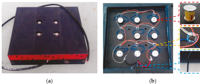
Figure 2. Illustration of the PEH: (a) outward appearance; (b) internal structure.
