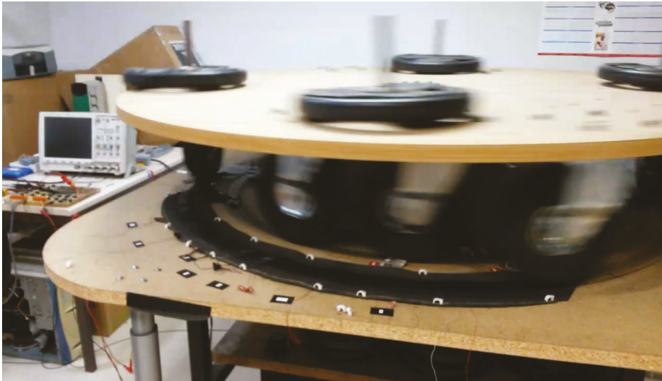
Figure 2. Piezoelectric characterization system in action.
