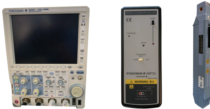
Figure 4. Yokogawa scope, voltage probe and current probe that are used for the data acquisition.
