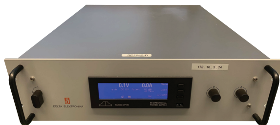
Figure 3. SM 500-CP-90 bidirectional power supply from Delta Elektronika, which is used to emulate the power electronic converters in low voltage dc grids.
